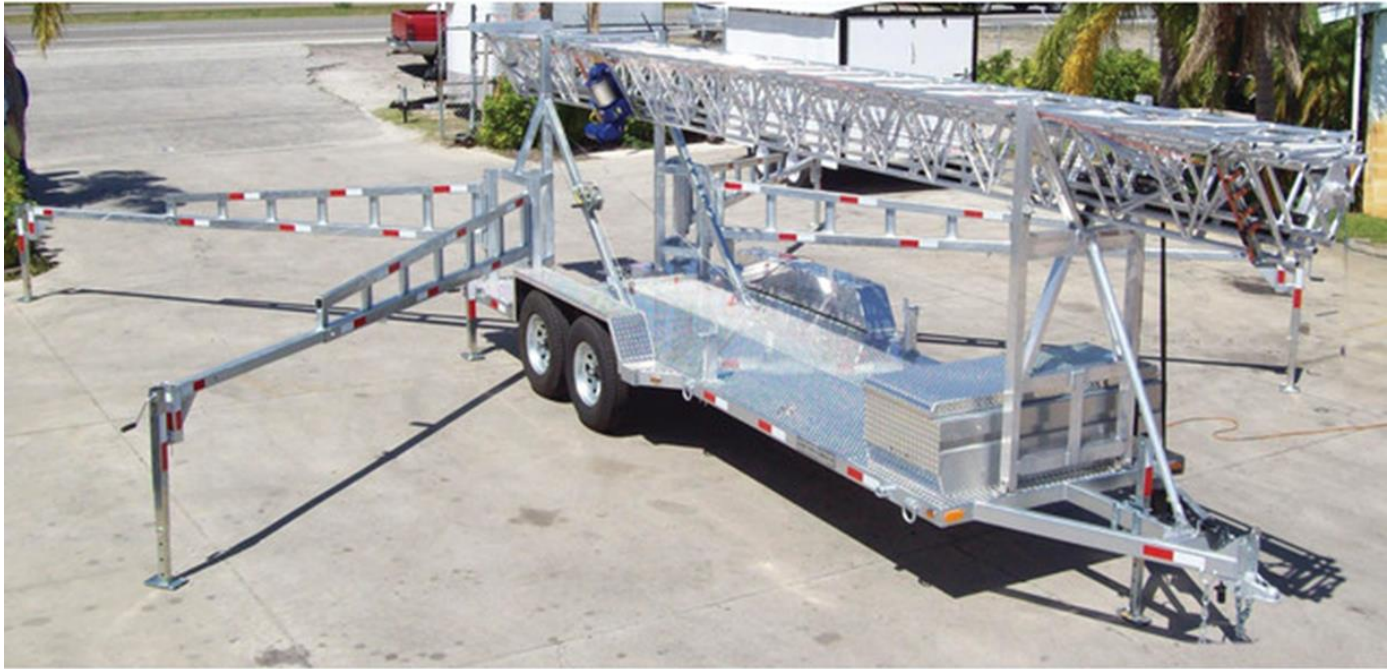
Figure 12 PEAK + Trailer with 109-foot tower
