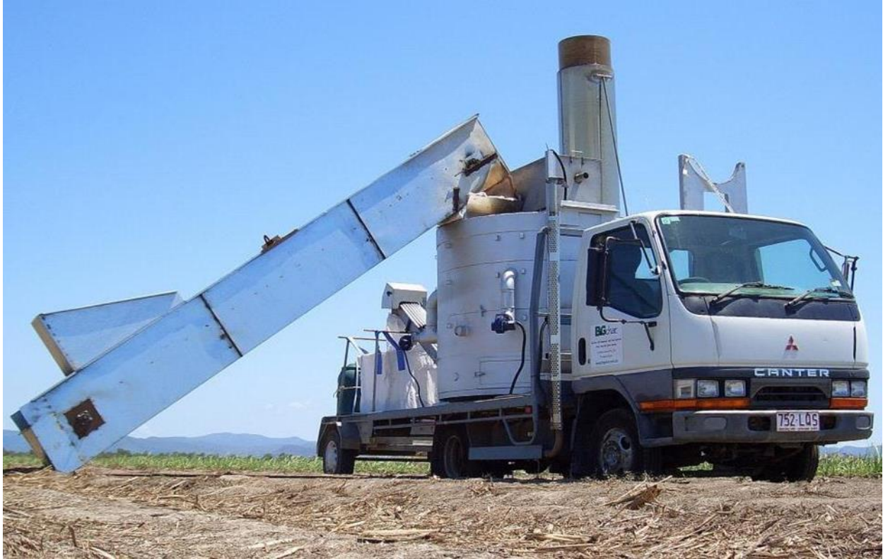
Figure 3, mobile Bio Char system that produces Power and Fertilizer from Biomass
