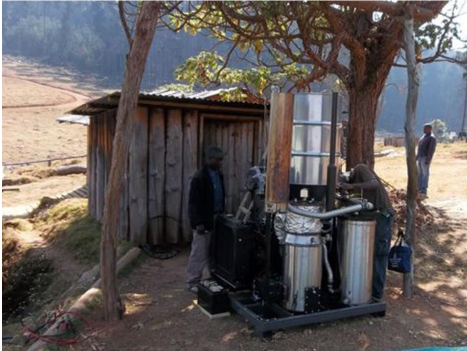
Figure 2, an 18KWH Power Pallet system that produces power from biomass
